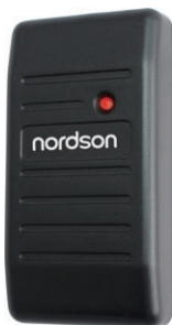
Model: NK-RF90S-HID Reading Range: 5-375px Communication Distance: WG≤100M, RS485≤1200M Dimension: 80*48*12.5(mm) Weight: 0.12kg
