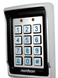
Model: NT-106 2n relay outputs 4-Operation Mode Card Capacity: 1000 Users Wiegand Signal: Input Dimensions: 120*76*37mm Gross Weight: 0.52kg
