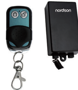
Model: NF-R16 Contact Output: NONCCOM Transmitting Freq: 433.92MHZ Remote distance: 15m Suitable for: access control Transmitting Distance: ≥70m (in open area) Dimensions: 66Lx45Wx30H(mm) Weight: 0.2kg
