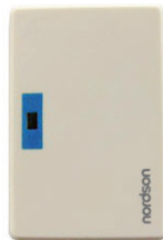
Model: GC1 Directional Active RFID Card Size: 90*60*8(mm)
